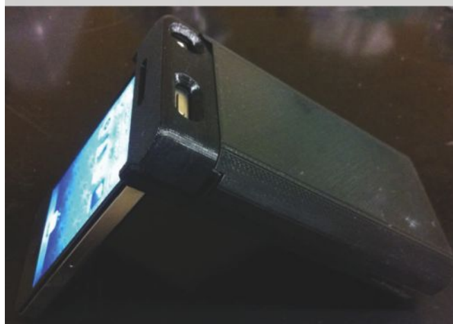
The optical detection components of the LOC system can be replaced with a single smartphone.
