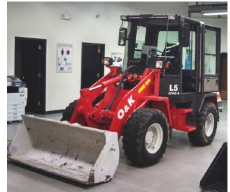
Prototype test vehicle with DC steer-by-wire system.
