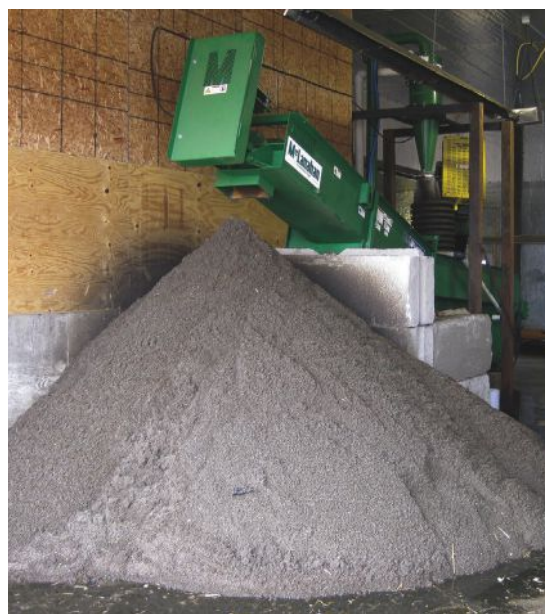
Recycled sand from a self-cleaning sand lane, Schwab Dairy, Delevan, N.Y.
