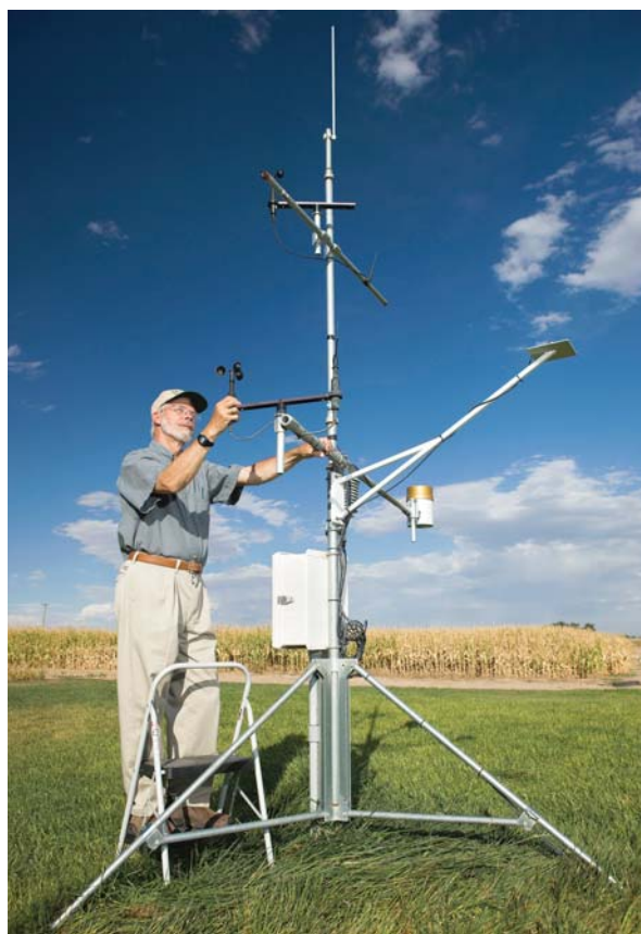
Tom Trout checks instruments on a weather station that predicts water consumption through soil surface evaporation and transpiration through plant leaves.
