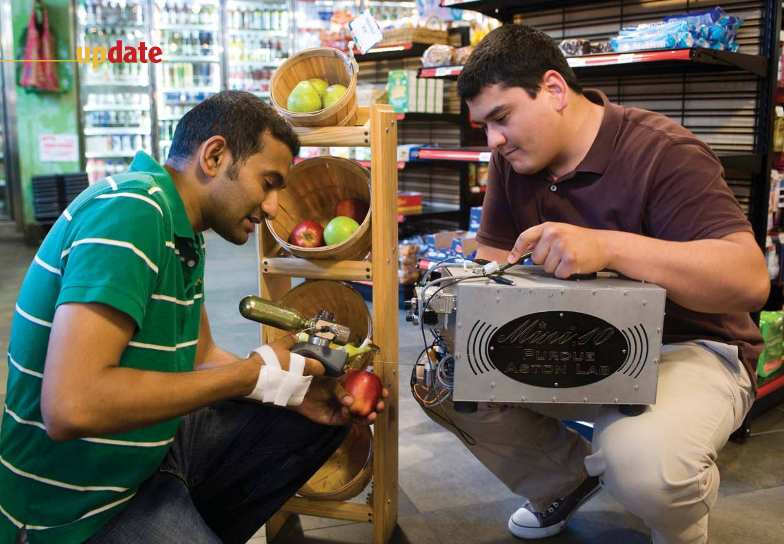
Santosh Soparawalla, left, and Fatkhulla Tadjimukhamedov demonstrate the miniature mass spectrometer used to detect chemicals on store produce. Photo by Mark Simons, courtesy of Purdue News Service.
