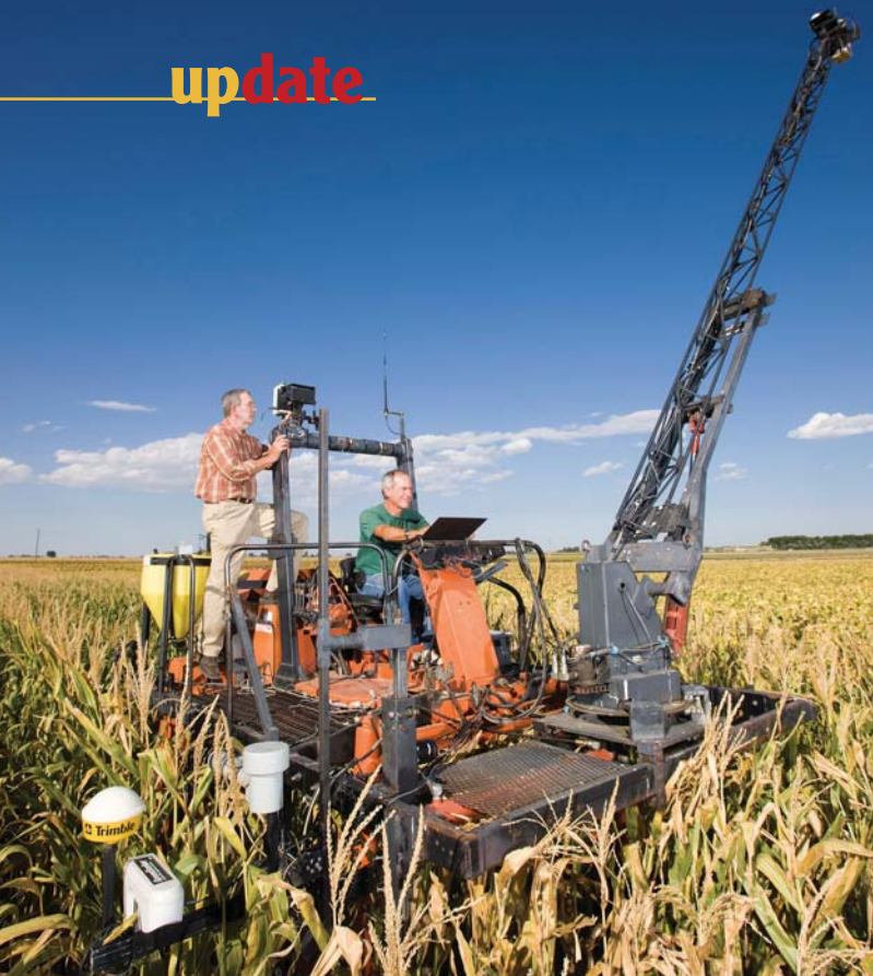
Walter Bausch (left) and engineering technician Ted Bernard measure reflectance, canopy temperature, and ground cover of corn with their mobile platform. The wheels of the platform roll between the rows of fully mature corn, while the sensors on the end of the telescoping boom look down on the crop from 4.6 m (15 ft) above the canopy.
